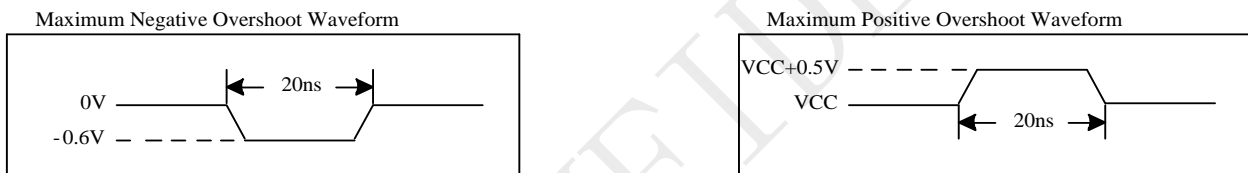
Figure 5-1 Maximum Overshoot Waveform
