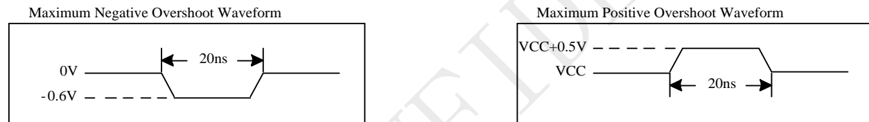
Figure 5-1 Maximum Overshoot Waveform
