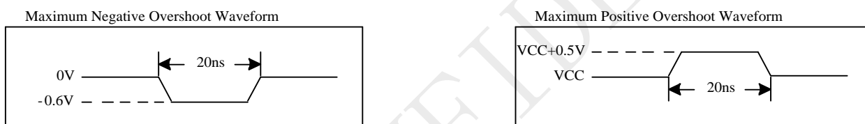
Figure 5-1 Maximum Overshoot Waveform
