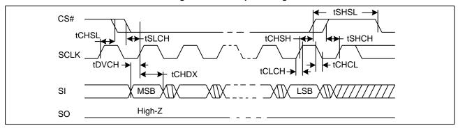
Figure 21. Output Timing
