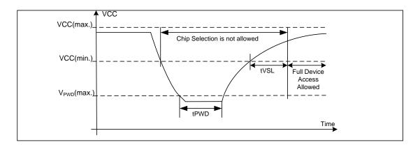
Table3. Power-Up Timing and Write Inhibit Threshold
