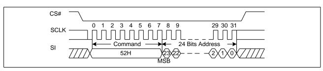
Figure 10. 32KB Block Erase Sequence Diagram
