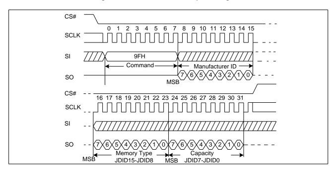
Figure 17. Read Identification ID Sequence Diagram
