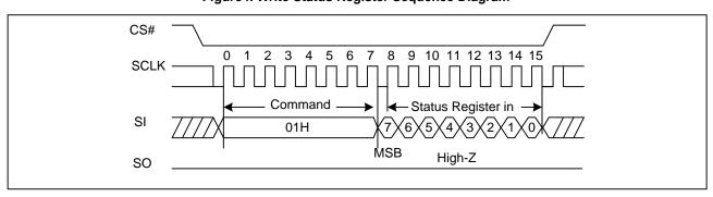
Figure 4. Write Status Register Sequence Diagram
