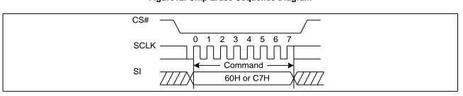
Figure 12. Chip Erase Sequence Diagram
