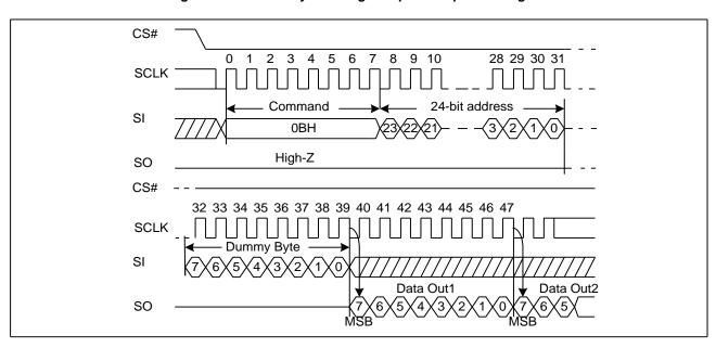
Figure 6. Read Data Bytes at Higher Speed Sequence Diagram
