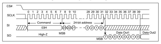
Figure 5. Read Data Bytes Sequence Diagram
