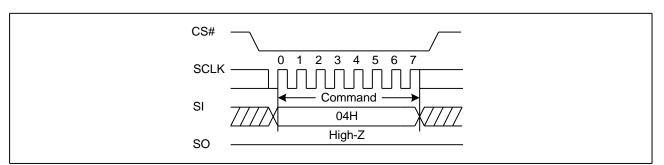
Figure 2. Write Disable Sequence Diagram
