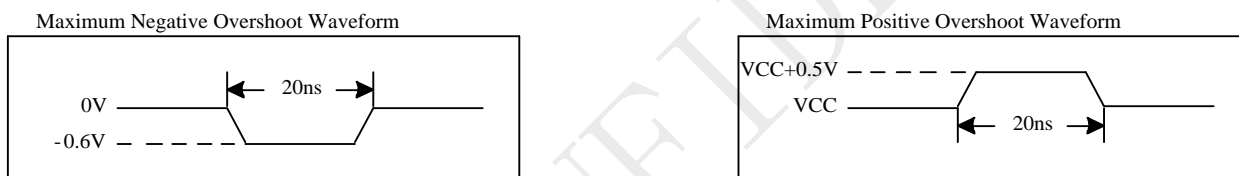
Figure 5-1 Maximum Overshoot Waveform
